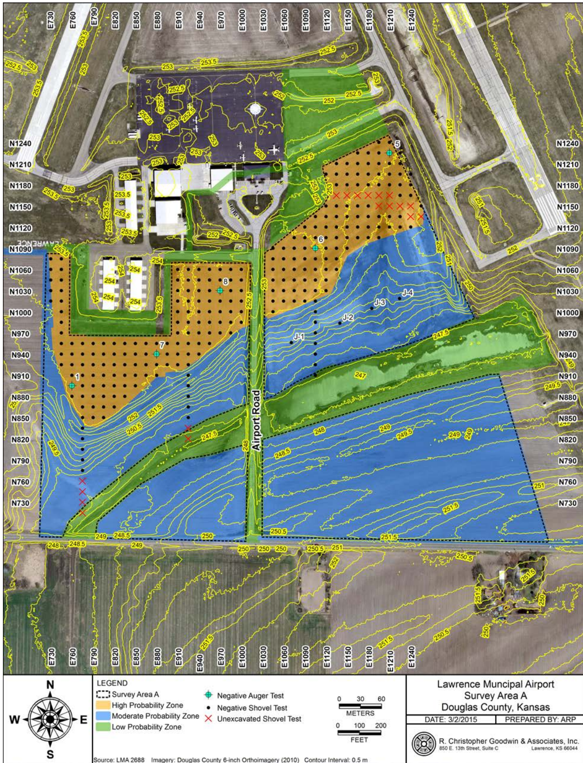
Figure 6.1. Phase II investigations of Area A.
