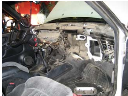
Heater core replacement, S-10
