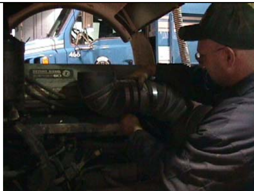
Tim Hays adjusting the air intake on a fire truck.
