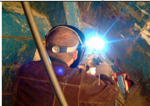
Jim Sparkes welding a wear plate in the hopper of a rear load refuse truck.
