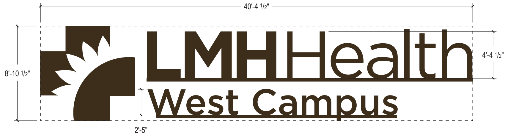
B Type 1D - Sign Detail scale: 3/4" = 1'-0"
