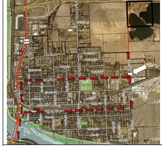
**Figure 4.** Proposed truck route shown with red arrows. Dotted lines show route past the gate on E 1550 Road. White line is a gate on E 1550 Road/N 9<sup>th</sup> Street.
