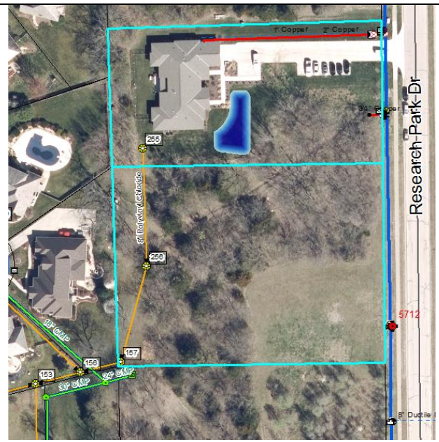
Figure 2b. Existing infrastructure; gold= sanitary sewer, blue & red=water, green = stormwater. (aerial does not show the second building that was built later)
