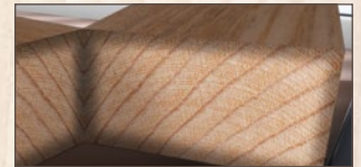
Traditional treatments only protect the outer surface
