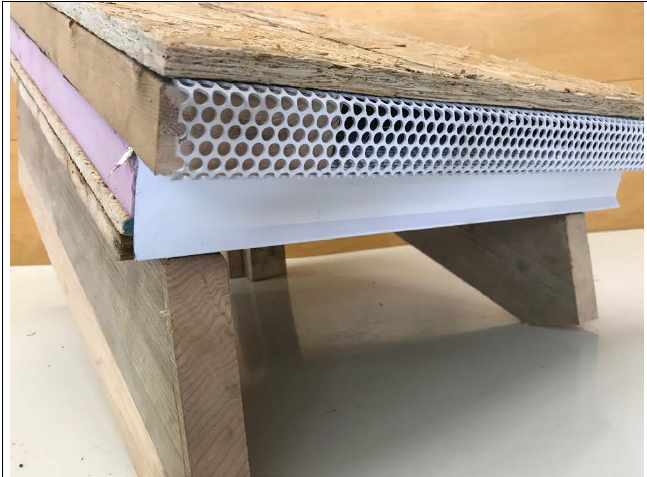
Mock-up with Rafter, Tongue and Groove, OSB, Rigid Foam Insulation, Air Space, and OSB
