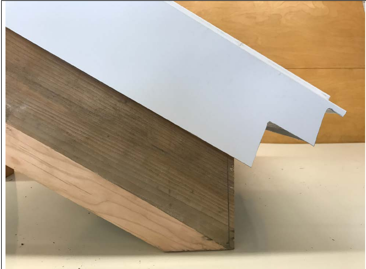
Mock-up with Rafter, Tongue and Grove, OSB, Rigid Foam Insulation, Air Space, OSB, and Metal Roof with Metal Trim
