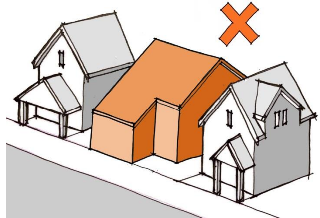
The illustration above reflects a building that does not reflect the forms of the structures adjacent to it.
