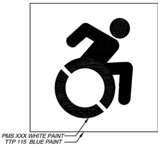
PAINTED HANDICAPPED PARKING SPACE & SYMBOL NOT TO SCALE
