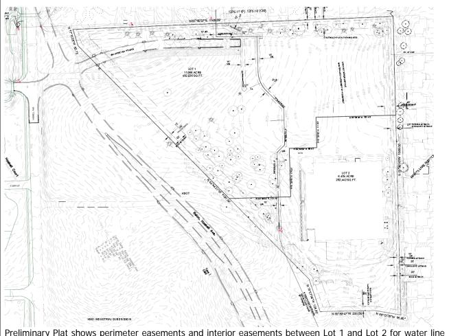
Preliminary Plat shows perimeter easements and interior easements between Lot 1 and Lot 2 for water line extension and sanitary sewer extension into Lot 1.
