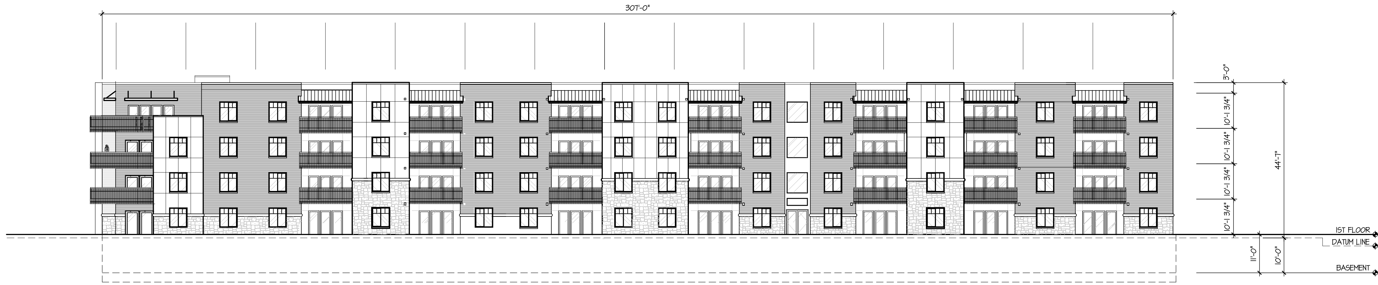
1 APARTMENT BUILDING SOUTH ELEVATION, POOLSIDE SCALE: 1/16" = 1'- 0"
