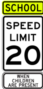
Figure 3. School Speed Limit Assembly
