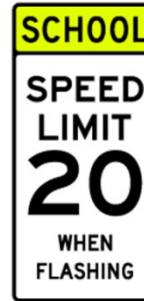
Figure 4. School Speed Limit (S5-1)
