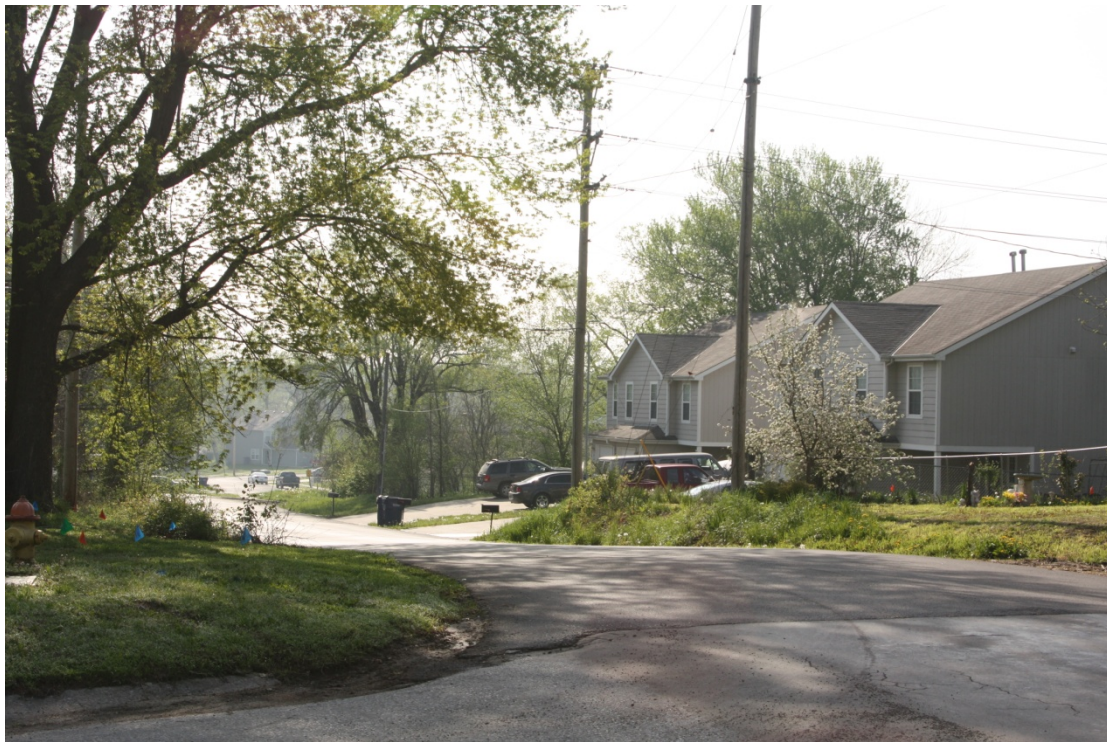
Figure 2. Neighborhoods to the west of Eudora Elementary School are primarily characterized as roads with no curbs, gutters or sidewalks. There are roads with sidewalks present to the west, but sidewalk connectivity toward the Elementary School is quite limited.
