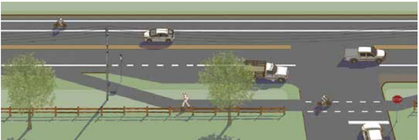
Figure 2.3: Shoulder Bikeway Crossing Transition to Separated Bike Lane or Shared Use Path
