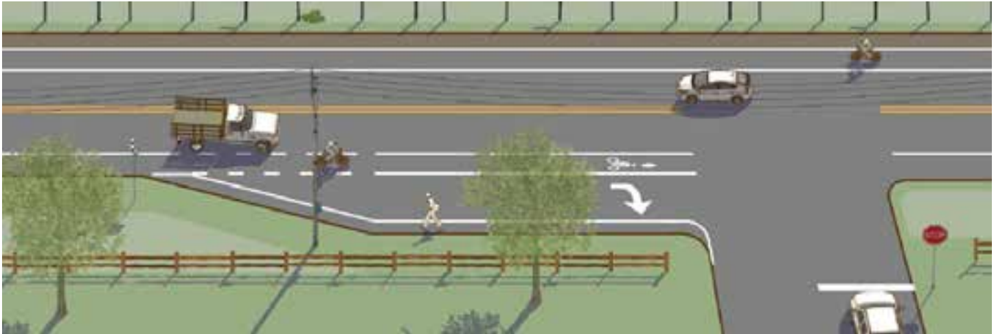
Figure 2.2: Shoulder Bikeway Crossing Transition to Bike Lane
