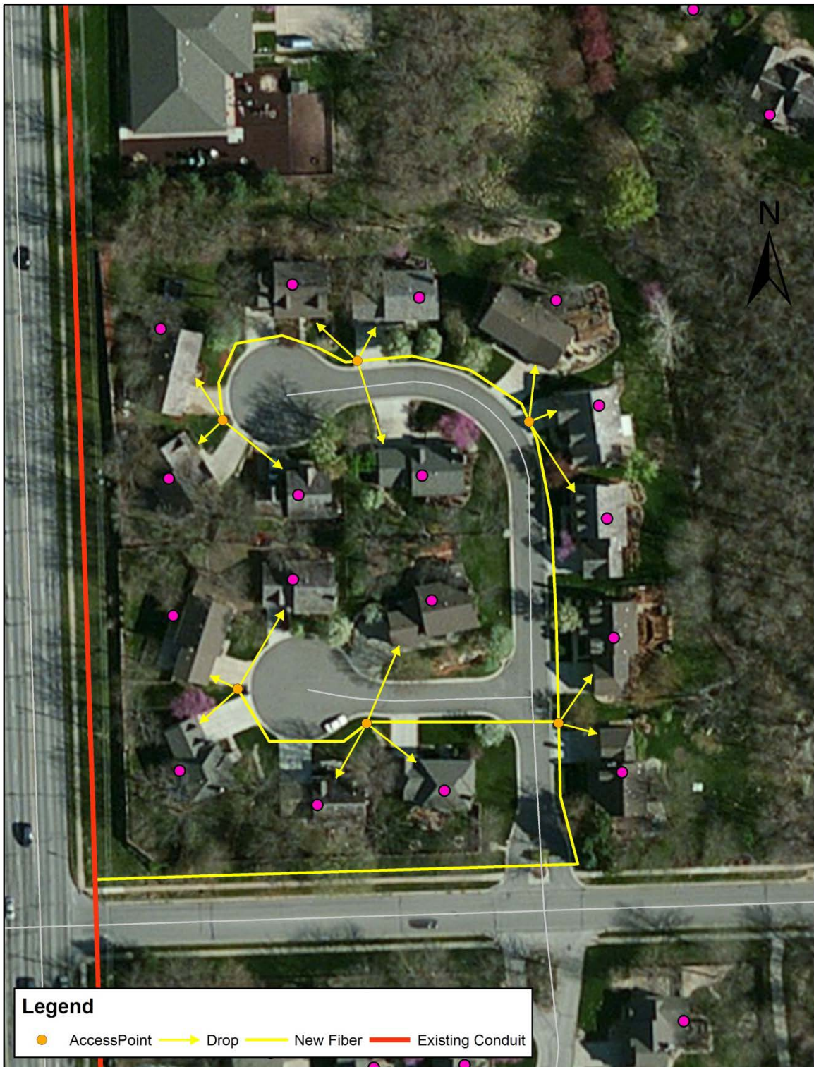
Figure 23: FTTP Distribution Design
