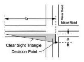
a = 28 ft (hand-measured distance)b = 335 ft (design standard)Not drawn to scale
