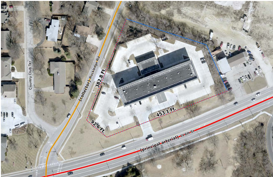
Figure 2: Street Designation for Frontage along Hampton Inn (2300 W. 6th St.)
