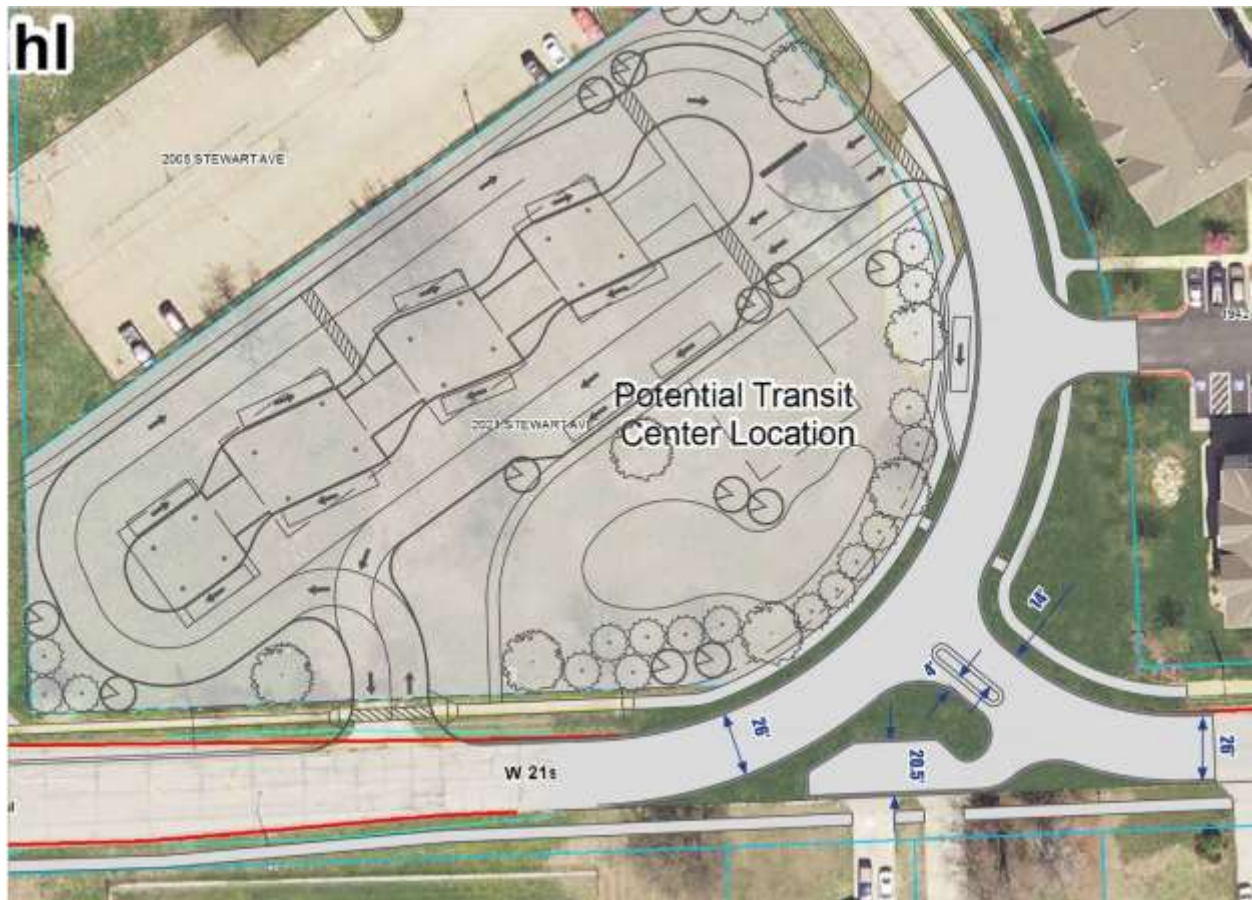
Figure 4 Final Concept Drawing: Realigned 21 st Street and Stewart Avenue Intersection with Traffic Diverter
