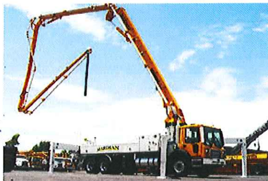
Figure 15. Concrete Pump Truck
