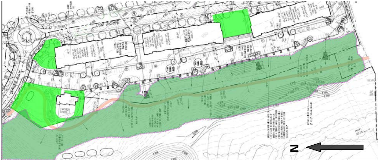
A note on the face of the plan states: "Trees on the west side of Lot 2 are to remain. If trees are removed or die a fence, wall or berm, per section 20-701 (H) will be provided with a Type 1 Byfferyard per section 20-1005 (D)"
