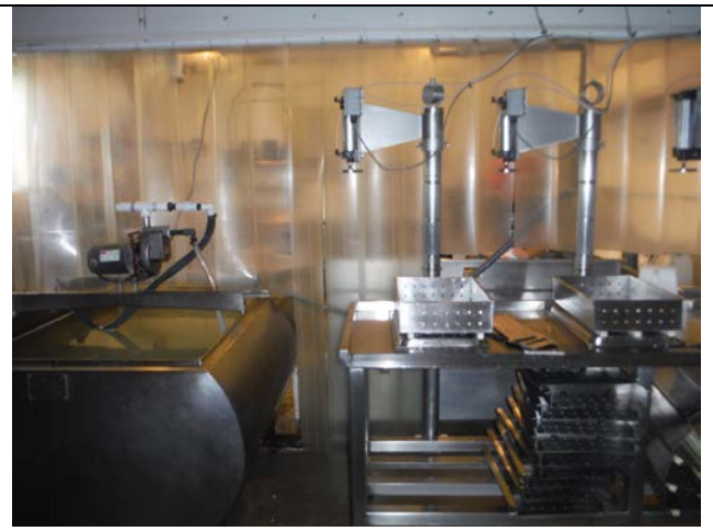
Figure 3b. Processing area for pressing the tofu.
