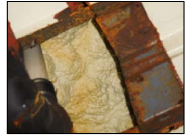
IAC rust from poor ventilation
