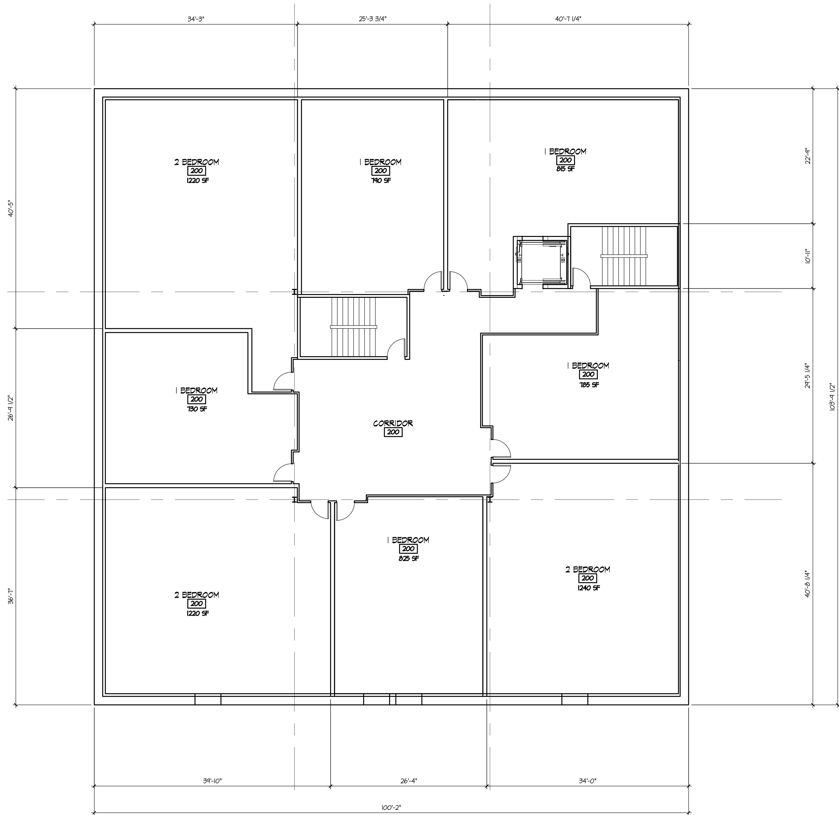
① 2ND FLOOR PLAN SCALE: 1/8" = 1'- 0"
