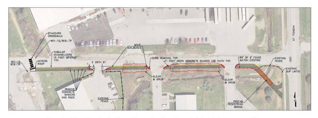
Notes: Install a 10 foot wide Shared Use Path adjacent to a 1 foot wide buffer space with tubular channelizing devices spaced 15 feet apart. A prefabricated pedestrian bridge provides access over the culvert to connect to existing shared—use path.
