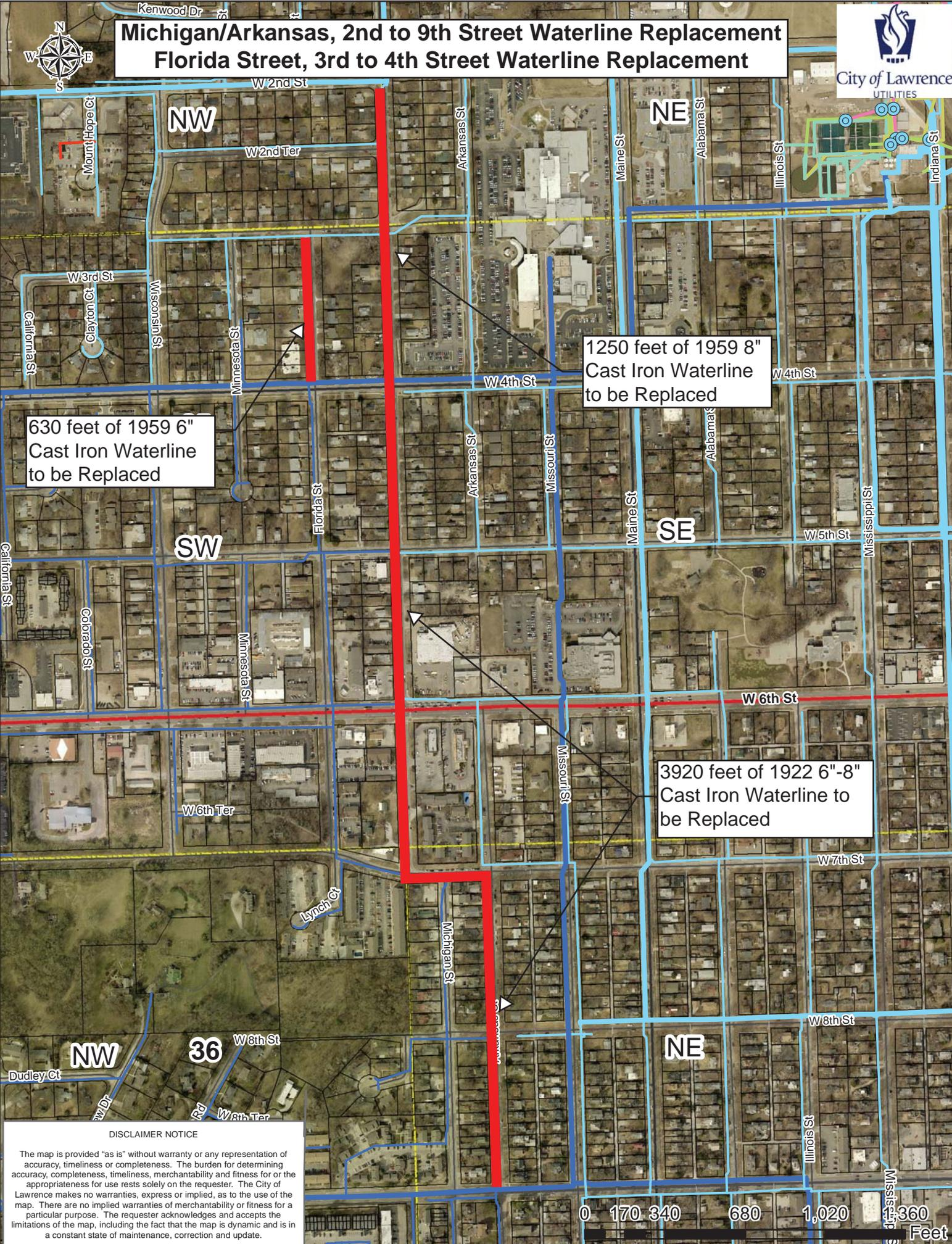
630 feet of 1959 6" Cast Iron Waterline to be Replaced
