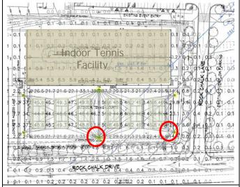
Figure 1. Site layout and lighting plan. Light fixture T3, bottom center and T6, bottom right, are circled.
