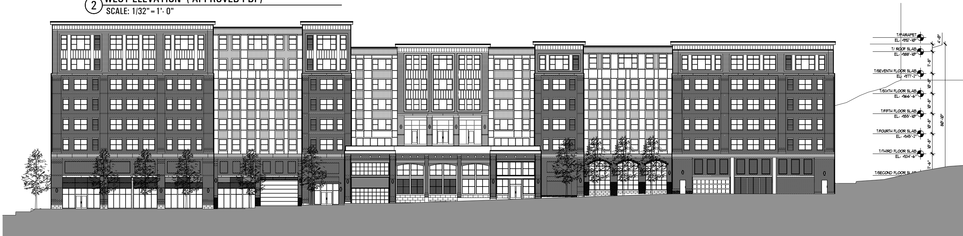
1 WEST ELEVATION (5/05/15) PROPOSED CHANGE SCALE: 1/32" = 1'-0"
