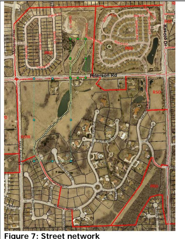
**Street Design:** The interior street network is proposed as a private street configuration. The Preliminary Development Plan is conditioned to provide a standard 27' street cross section. The plan currently shows sidewalks on only one side of the private street. Note 1.9 must be revised to also note the street width shall be 27'.
