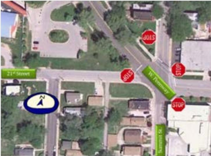
The 21<sup>st</sup> Street intersection at West Pennway Boulevard is also a non-standard intersection. The difference from the 17<sup>th</sup> Street intersection is that the 21<sup>st</sup> Street intersection has five-legs. West Pennway approaches the intersection from the north at a skew, while Summit Street, 21<sup>st</sup> Street, and West Pennway from the east all approach on a perpendicular grid.
