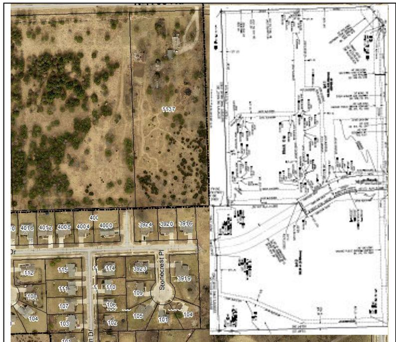
**Figure 1.** Plat overlaid on aerial photo showing right-of-way for future extension of Spring Hill Drive.
