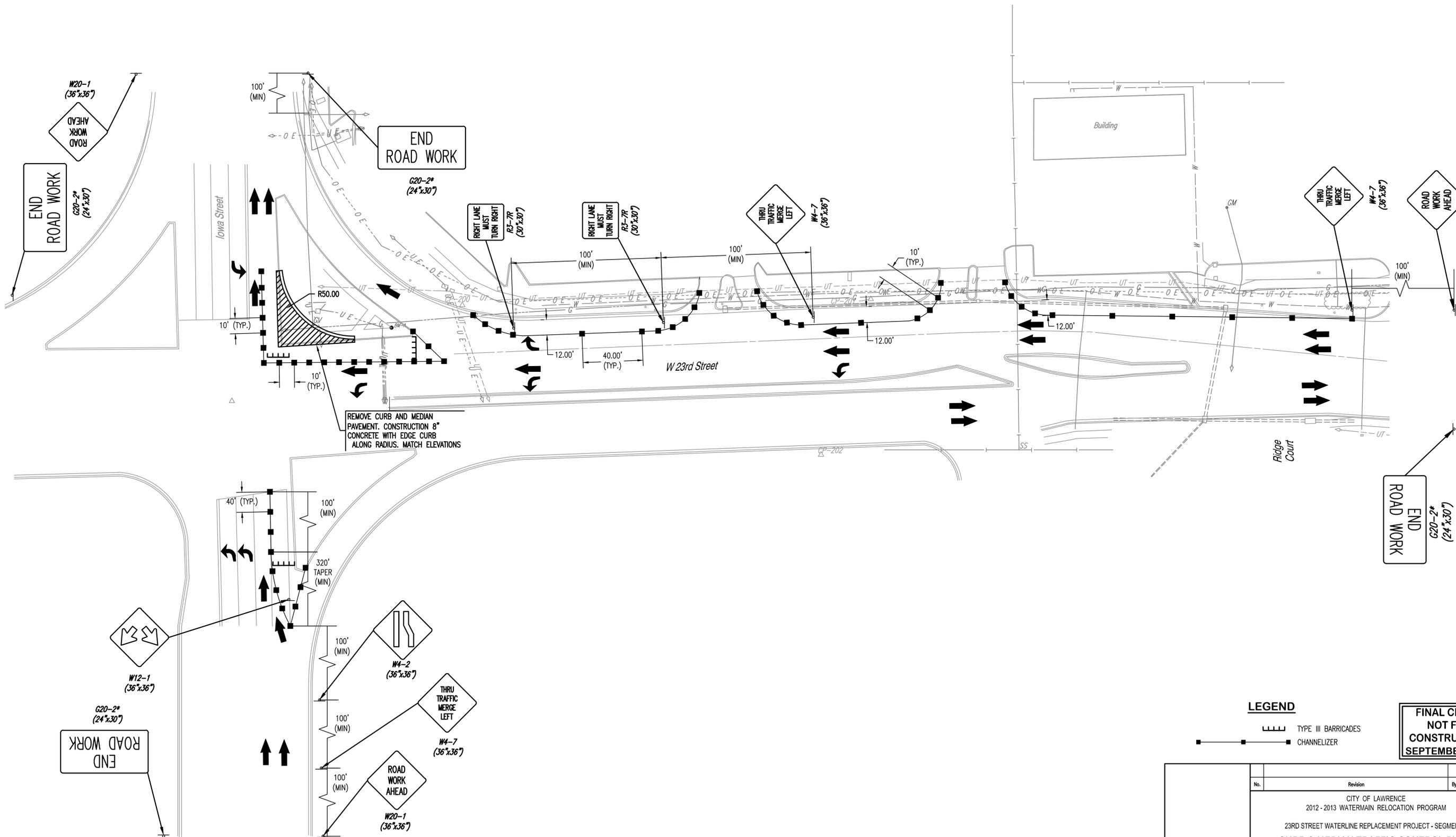
REMOVE CURB AND MEDIAN PAVEMENT. CONSTRUCTION 8" CONCRETE WITH EDGE CURB ALONG RADIUS. MATCH ELEVATIONS
