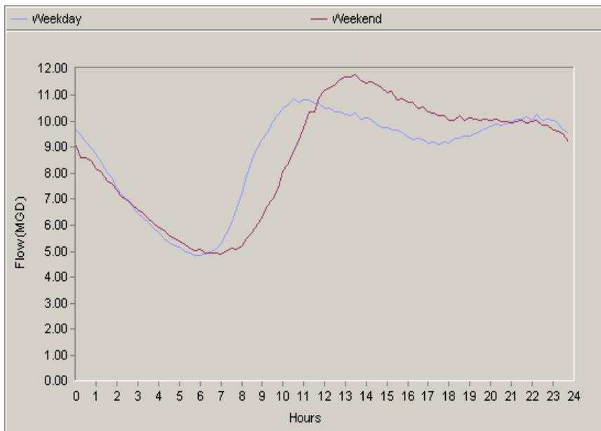
**Figure 2.7. Diurnal Curves - Wastewater Treatment Plant**
