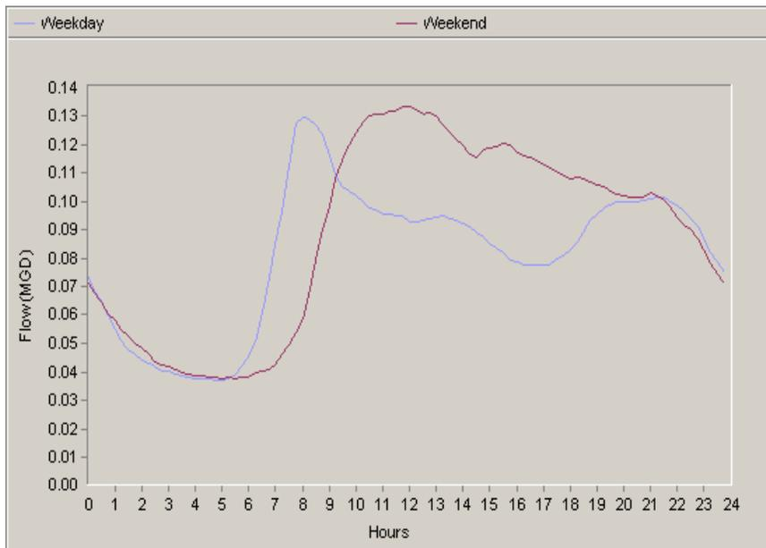
**Figure 2.6. Diurnal Curves - Flow Meter BC1 003**
