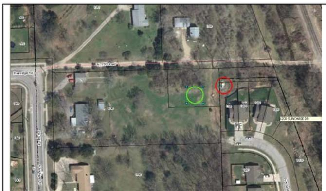
**Figure 1.** Current and proposed location of Pump Station 25. Existing location in red, proposed in green.
