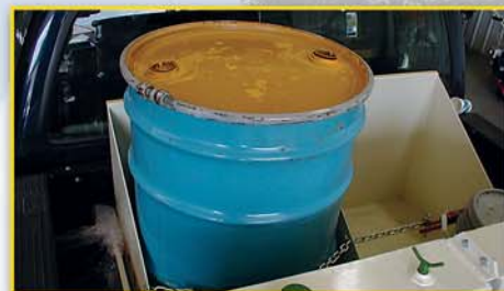
Drum tie-down in lieu of (2) 60 gallon tanks, allows painting directly from drums.
