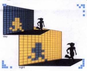
Last spring, students from KU's Industrial Design program created a proposal to develop and install a wall of tiles which respond to movement within the tunnel. Each tile will be lit with blue and orange LEDs that use IR sensors to respond to motion.
