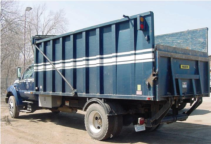
The Bulk Truck collects scheduled pick ups of items that are too large to fit in the Rear Loader unit, and items left at Front Loader locations that will not fit into containers.
