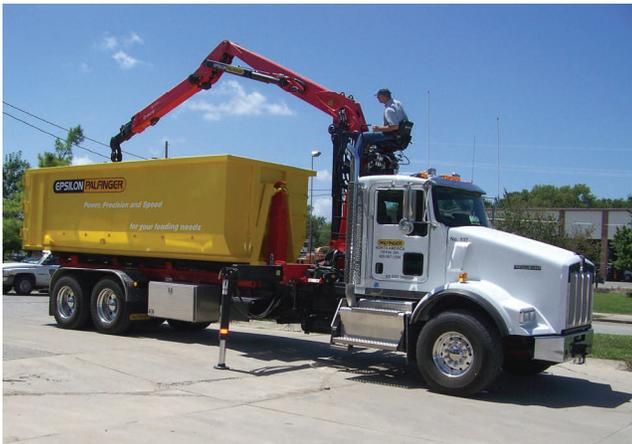
The Division demoed different styles of bulk trucks. The vehicles had a telescopic crane arm that could reach items as far as 32 feet from the truck and then deposit them into the container.
