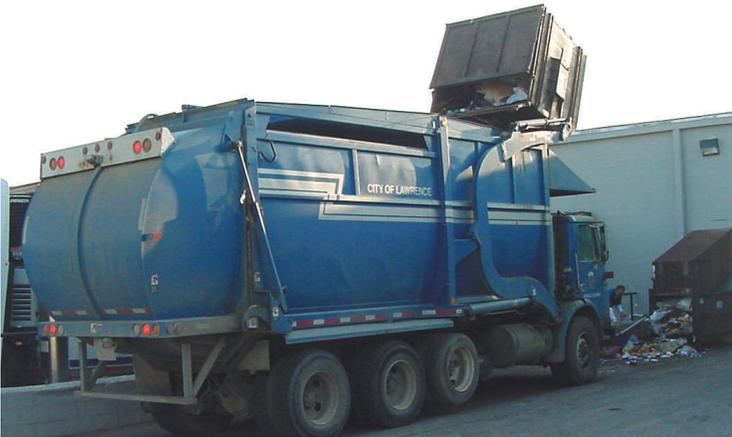
Front Loaders provide fully automated commercial services for 4 to 10 cubic yard containers.
