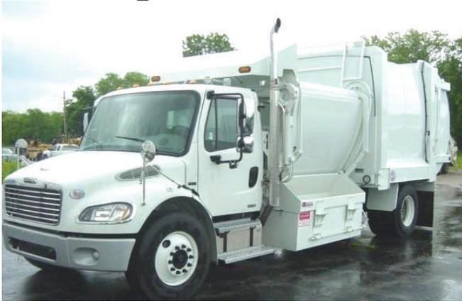
The Division demoed a semi-automated side loader. The unit has low entry cabs with 1 yard buckets on each side that can load four, 90 gallon containers at a time.
