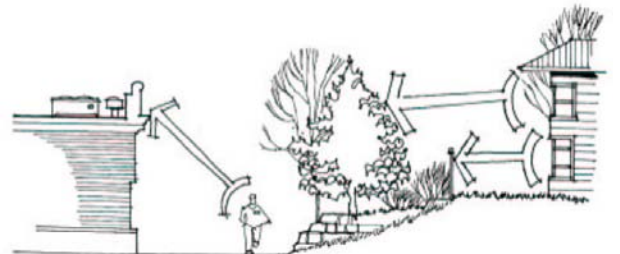
example showing how rooftop equipment can be screened & remain out of view from the public or adjacent properties
