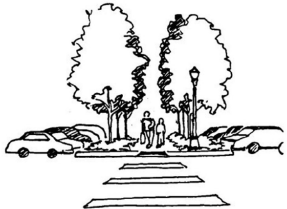
to improve pedestrian safety & security, walkways must be clearly defined where they cross a drive aisle or parking area
