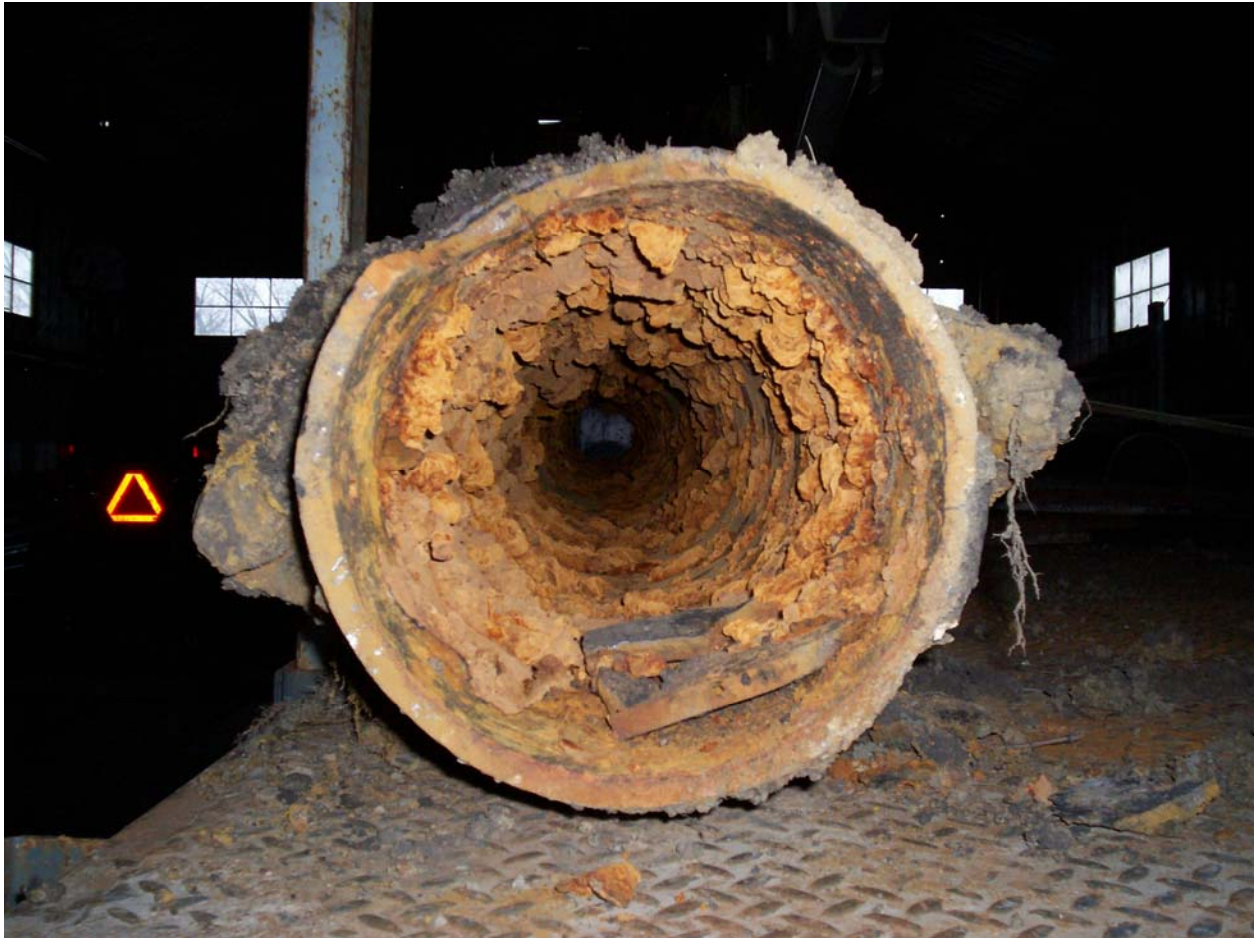
Section of Existing 1922 10" Watermain From 2005 Main Break – 1700 Block of Kentucky
