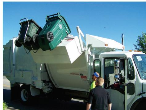
These units were used on both yardwaste and residential routes. The truck's ability to make single sweeps down a street increases route efficiency, eliminates back tracking, wear on equipment, and city right-of-ways. The drawbacks identified in the use of this type of equipment in Lawrence operations are that additional work is transferred to the bulk truck and it cannot capitalize on the efficiencies of integrated residential / commercial routes for rear load dumpsters.
