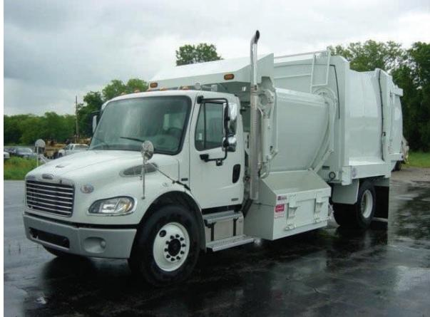
The Solid Waste Division has recently looked at semi-automated equipment from Elliott and Downing. The Units are low entry cab trucks with 1 yard buckets on each side of the body that can load 4-90 gallon containers at one time into a 3 yard hopper in the center of the Unit. The stand up dual drive capabilities makes the operations of loading and driving safer and less strenuous on the Operators.
