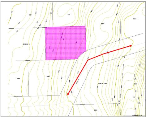
**Figure 1.** Purple highlighted area is the subject property. Distance of street section marked with the red arrow is approximately 272 ft. The change in elevation is 20 ft (the bold contour lines mark 10 ft change in elevation).
