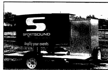
Sportsound 1000 trailer mounted option with onboard generator
