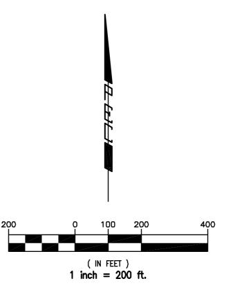
Basis of Bearings is N 87° 42′26″ E on the north line of the NW 1/4, Sec. 13, based on the Kansas State Plane Coordinate System, NAD83, North Zone
