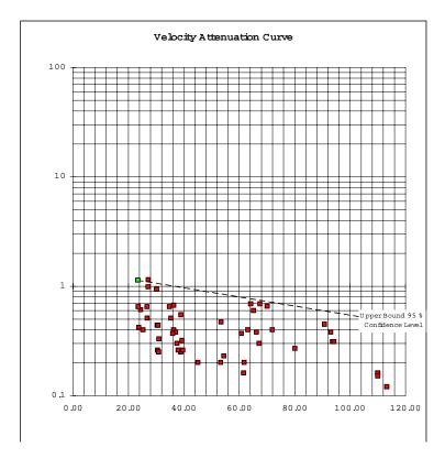
Utilizing the techniques of regression analysis and the vibration prediction formulas, blasts can be optimized and designed with confidence for close-in or tight blasting. The added benefit of high frequencies helps to reduce the potential of vibration effects and damage.
